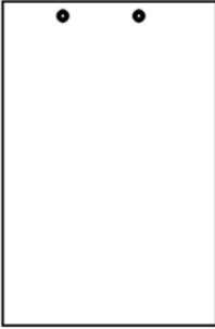
2 File Hole Punch Top 5/16" Holes 2-3/4" Center-To-Center
